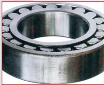
Trace caused by sliding between housing diameter and bearing outside ring
