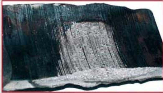
Adhesions occur due to the heat from the surfaces of shaft and bore
