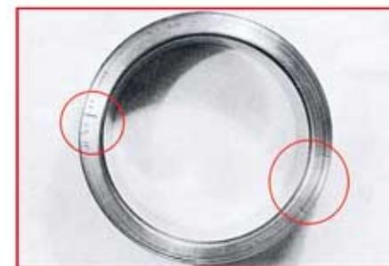
Cracks occur due to the heat generated by friction between inner face and shaft shoulder
