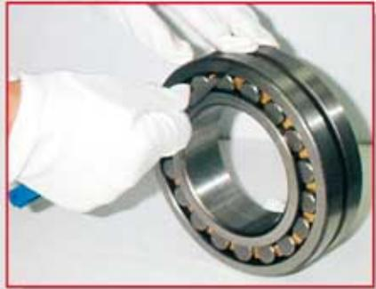
The arithmetic mean value of minimum and maximum is the radial clearance. If the each row's clearance is qualified, get the arithmetic mean value of the two rows as bearing's clearance.
