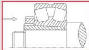
Bearings located using extraction sleeves are dismounted with the aid of the extraction nut.
