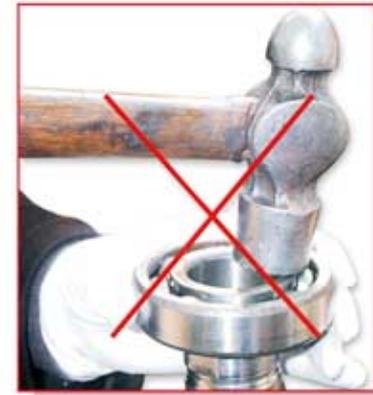
Broken rib knocked by hammer
