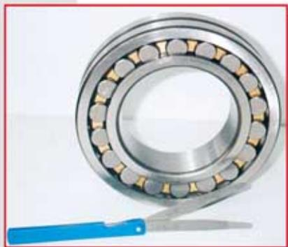
**Radial internal clearance in spherical roller bearing Units:( $\mu\text{m}$ )**
