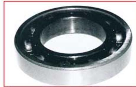
The bearing surface has changed into black after being heated by acetylene gun.
