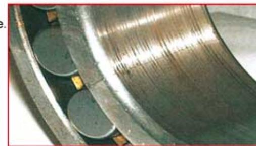
The sliding track between shaft and bearing bore
