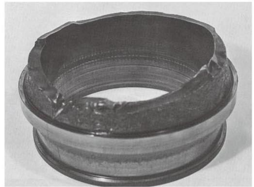
Figure 14 POOR SEATING ON TAPERED SHAFT
