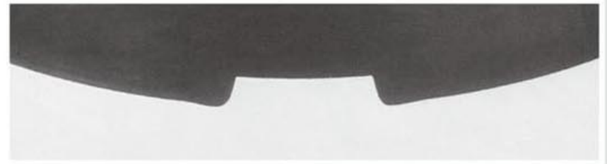
Figure 30 ABRASIVE WEAR — OUTER RING CROSS-SECTION
